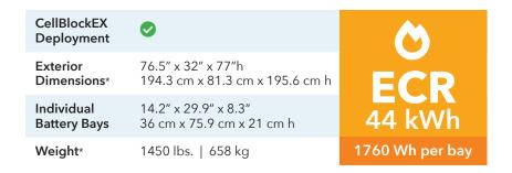
ECR = Energy Containment Rating. This calculation is the result of validation testing.
