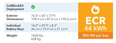
**ECR = Energy Containment Rating.** This calculation is the result of validation testing.
