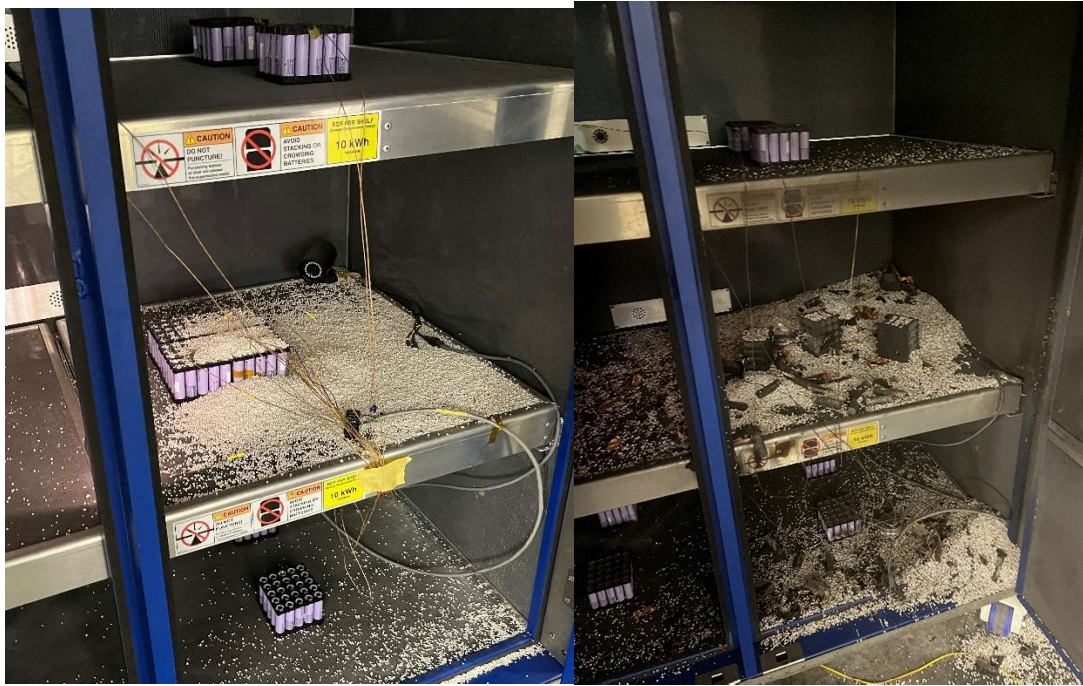
Figure 12 – Post-test interior of the cabinet after Test 1 (left) and Test 2 (right)
