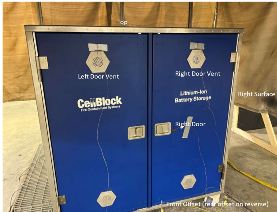
Figure 8 – Location of exterior thermocouples on CellBlock XL Cabinet
