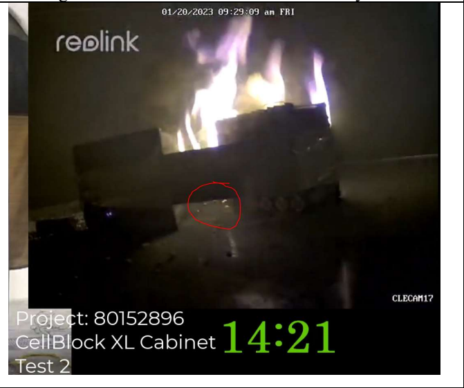
First visible CellBlockEX released away from camera side of packs
