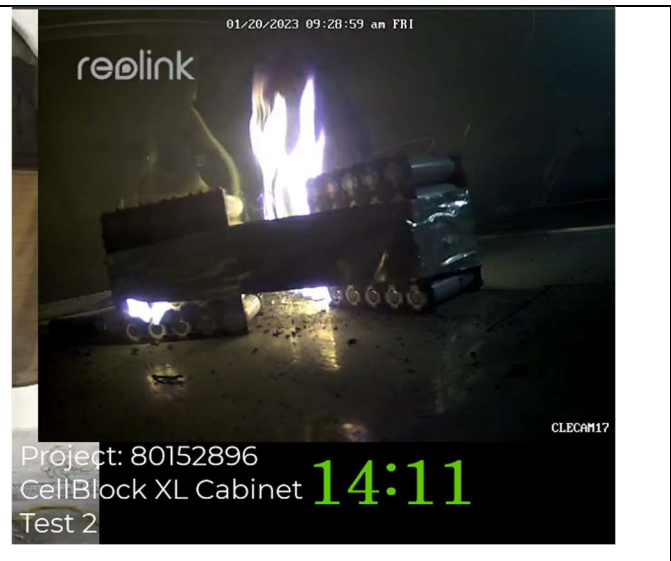
Flame growth after initial after thermal runaway events
