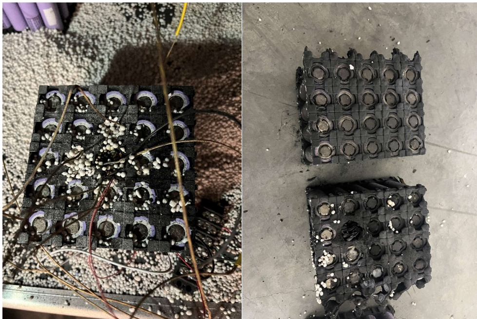
Figure 13 – Post-test condition of the initiating pack in Test 1 (left) and Test 2 (bottom right)
