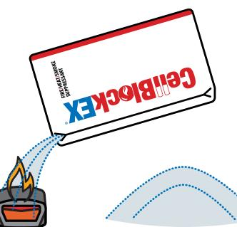
Dispense CellBlockEX on battery at source of flame or smoke.
