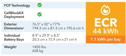
**ECR = Energy Containment Rating.** This calculation is the result of validation testing.
