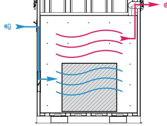
EMS series provide active temperature monitoring and regulation
