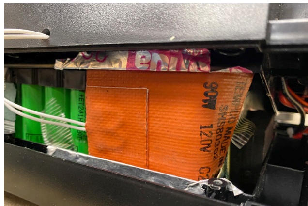
Pre test - test sample assembly with 90 watt heater tape attached.
