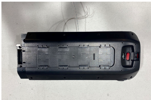
Pre test - test sample, thermocouples attached.
