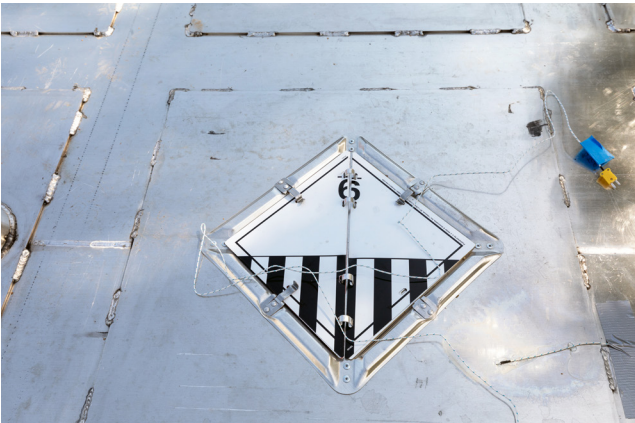
Case top pre-test. Thermocouples attached.
