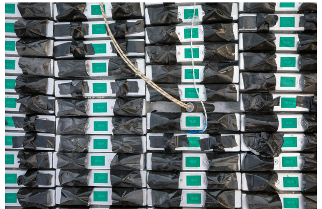
Test sample pre-test, showing placement of cylindrical heater
