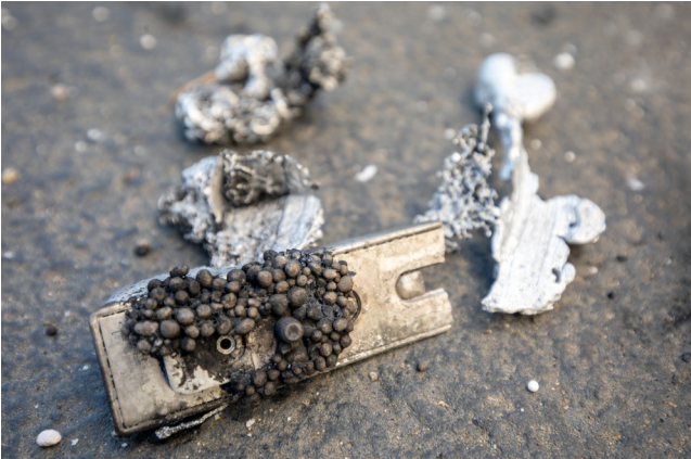
Post test - fused metal debris
