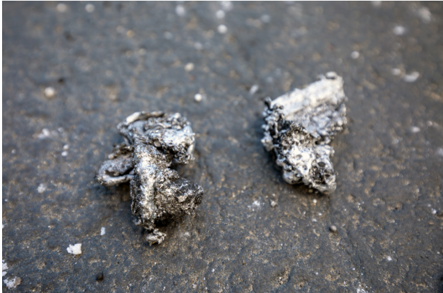
Post test - fused metal debris
