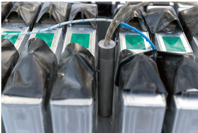
Test sample pre-test, showing placement of second cylindrical heater
