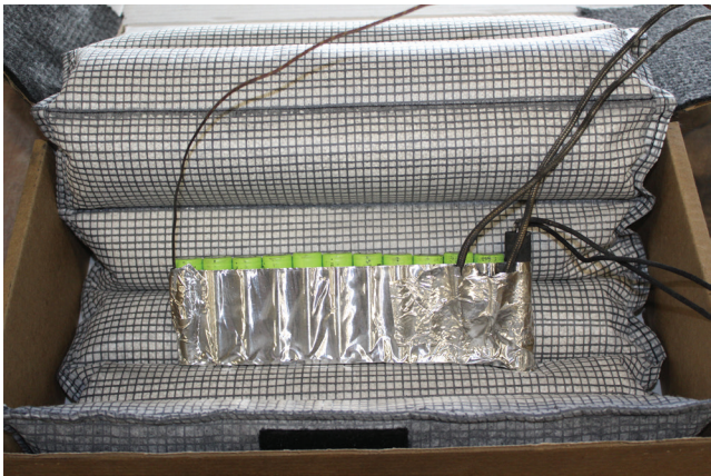
Battery assembly with thermocouples view in box
