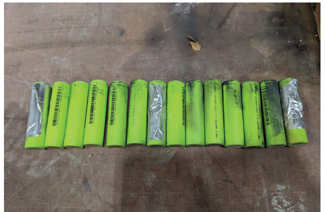
Unpropagated batteries post test - undamaged; no leaking electrolyte observed
