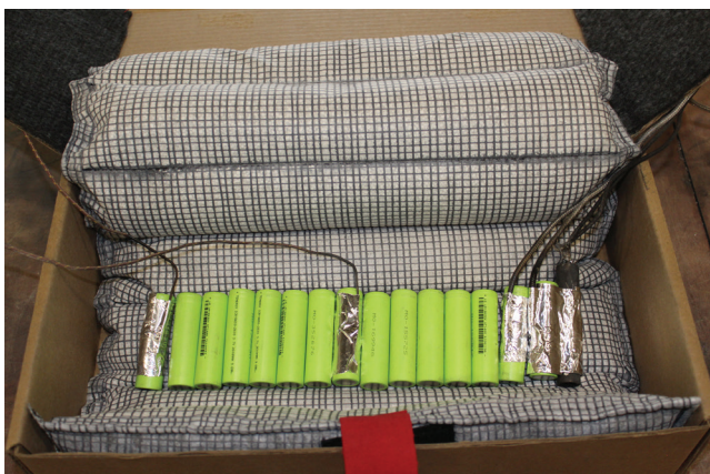
Inside view with battery assembly and thermocouples pre test
